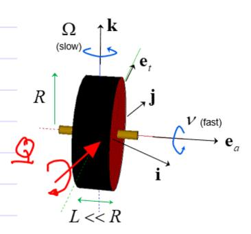
Example 6.8.2 A boomerang is subjected to an aerodynamic lift force and moment
