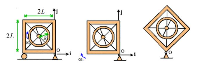
**Example 8.7.3** The figure shows a 1-D prototype for the 'Cubeli.' The frame has total mass *M*, the ring has mass *m*.
